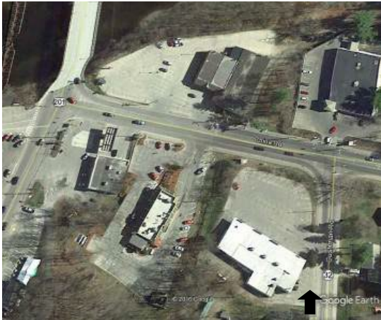
China Road (Route 137) from Bay Street (left) to Cushman Road. Midblock crosswalk striping is not visible (paint worn). (Image: Google Earth)
